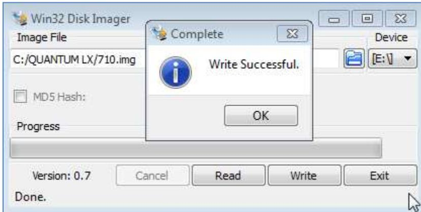
5). Click OK and Exit to complete image copy. Remove the USB Flash Drive. As with any USB device, be sure to select “Safely Remove Hardware” to stop the USB device, before removing the USB flash drive.
